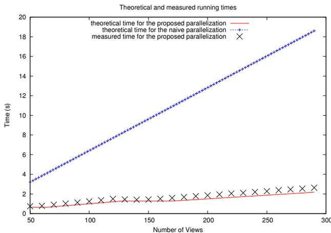
**Figure 5. Time spent by the naive and proposed parallelizations using 5 GPUs**
