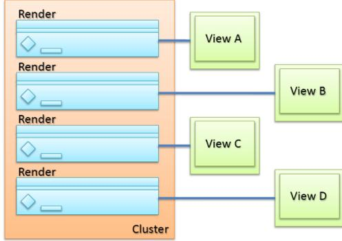
**Figure 1. Intuitive Architecture - The views are distributed among the available GPUs. Each GPU render the entire pipeline.**
