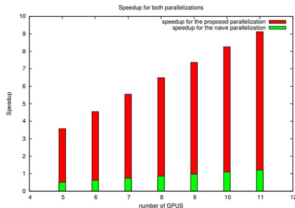
**Figure 7. Speedup of the naive and proposed parallelizations for a load of 1000 views.**
