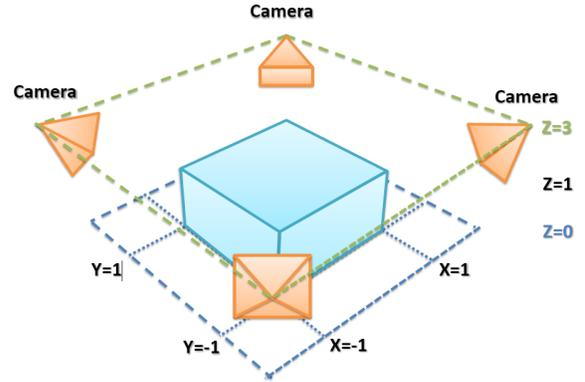
**Figure 3. Four cameras are used to sample each tile. The sample volume is delimited by the planes  $z = 0$ ,  $z = 1$ ,  $x = \pm 1$ ,  $y = \pm 1$**
