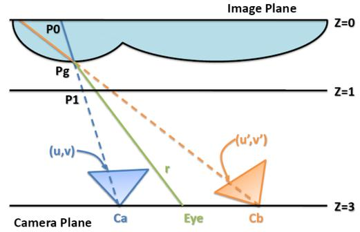
**Figure 4. Given ray  $r$ , we must find coordinates  $(u, v)$  and  $(u', v')$  which correspond to intersection point  $P_g$**
