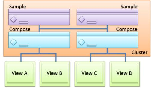
**Figure 2. Proposed Architecture - The pipeline is divided into sampling and compositing stages. The GPUs are assigned to each stage as a function of the number of views.**
