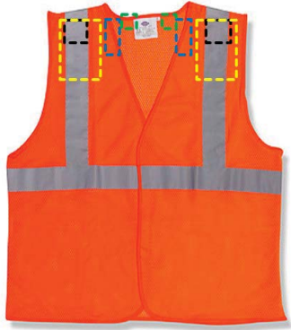
This picture shows the conceptual design for the vest. Colored squares show the approximate placement of output devices: Green and blue - vibrating motors; Black - speakers; Yellow - LEDs. The general placement stayed the same in the finalized vest.
